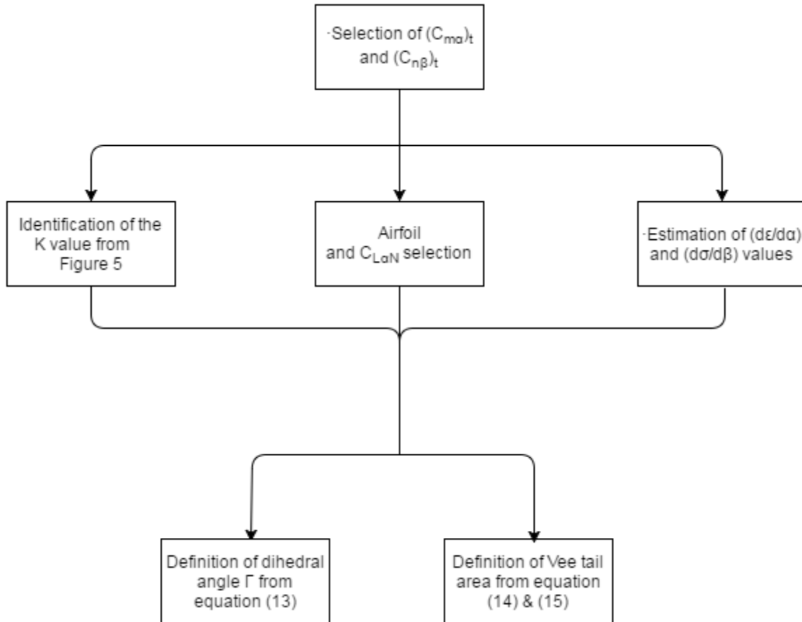
Fig 4: Vee-tail designing steps.
